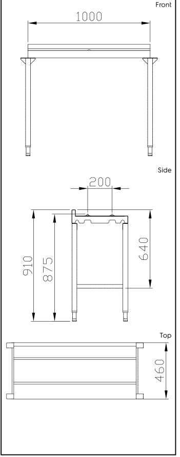
Handling System for Rack Type Cord Conveyor for Trays, Sorting Low Edge - 1000mm
